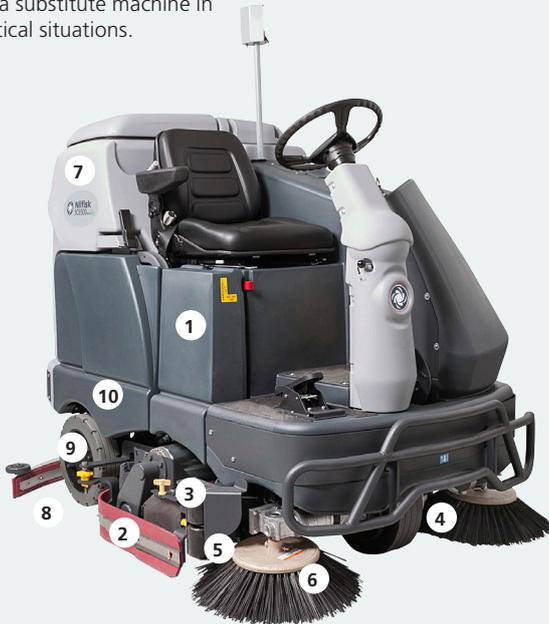
1. Ecoflex system provides customizable settings to save water and chemical
